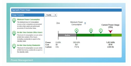
With real-time tracking, system administrators know exactly how much time an endpoint spends in idle, active, standby or off states resulting in an accurate view of current power usage and cost. Data can also be exported further analysis. Wake-On LAN capability, also provided by BigFix power management, helps deliver high first pass patch success rates by being able to wake systems that are powered off.
